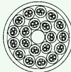
MS20-JP 20 jacketed and screened pairs x 0.22 mm 2 .
