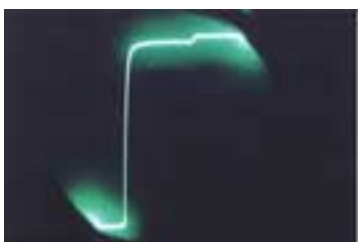
Pict. 4 shows response of RG179, a top-grade, 75 ohm coax made to US Military standard MIL-C-17D. Note that the two Supra cables perform similarly cleanly. Note also that all are fitted with 75 ohm BNC plugs.
