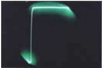
Pict. 1 shows reference with special GR-connected 50 ohm load, acting as a near pure resistance at all frequencies to above 2GHz (high RF).
